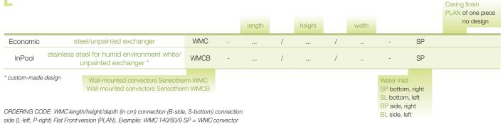
element, length 1400 mm, height 600 mm, depth 60 mm, bottom connection on the right side.
