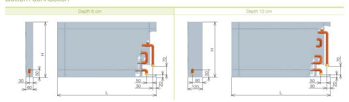
WMC is available in right or left version. The connecting side must be indicated in the order. In the schematic representations the dimensions are expressed in mm.
